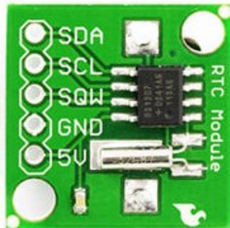
Illustration 18: A RTC module. Flexible jumper wires can be soldered to the board. This is the only situation where soldering is needed in the project. The SQW pin is not needed in this project. There is a link to the board on sparkfun: https://www.sparkfun.com/products/99
